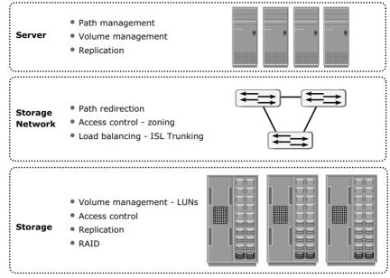
Figure 10-4: Storage virtualization at different levels of the storage environment
