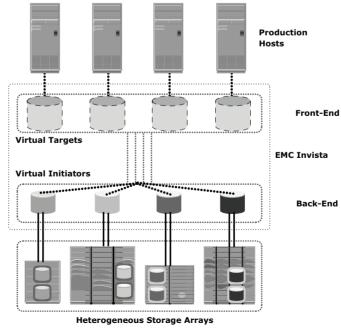
Figure 10-8: Storage virtualization with EMC Invista
