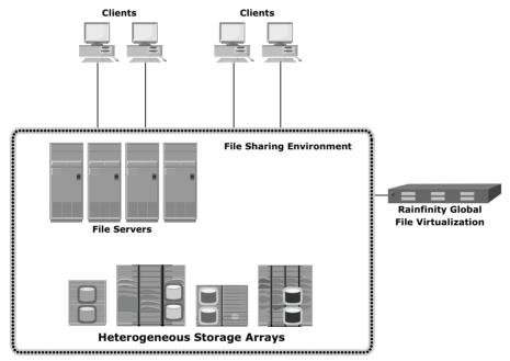
Figure 10-11: File-level virtualization with Rainfinity
