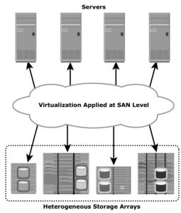
Figure 10-6: Block-level storage virtualization
